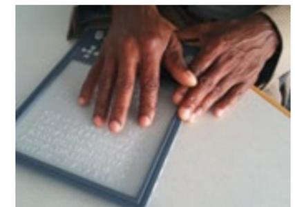
The BLITAB-Tablet generates lines in Braille instead of an LCD screen. It is currently tested by thousands of students.
